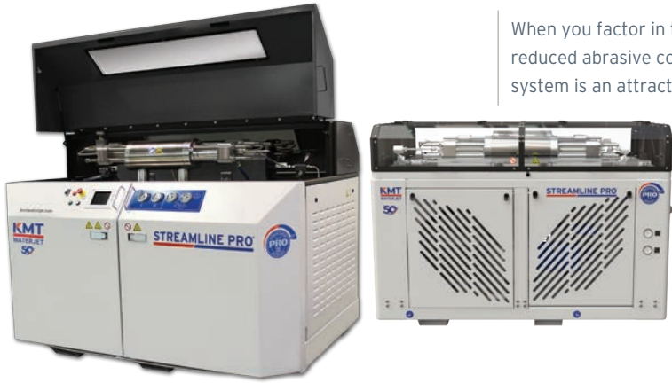
125hp/60hp Dual Head Cutting, Redundant Intensifiers
